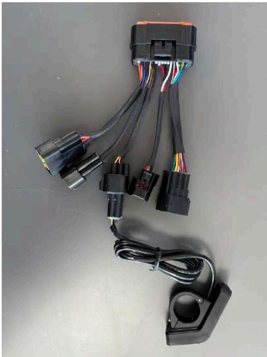
The Torp Display is being installed directly to the controller's wiring harness, as shown on the photo.
