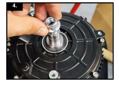
Remove the nut from the TORP motor.
