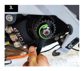
When everything is mounted, press the rear brake and tighten the nut (clockwise direction) a bit more to 40-50 Nm.
