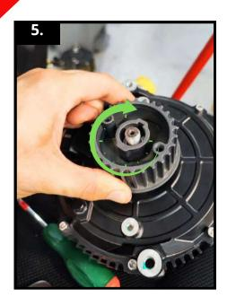
Mount the pulley on the shaft. The shaft key should be premounted on the shaft.
