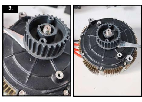
Remove the pulley with a lever, working a little from each side.
