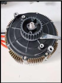
Remove the pulley with a lever, working a little from each side.
