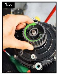
Mount the pulley on the shaft. The shaft key should be premounted on the shaft.
