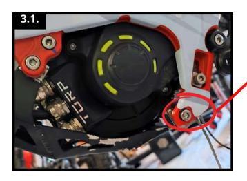
Usually the metal bashguard is mounted like this. However, in order to install the TM40 minor modifications are required.
