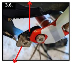
Lift the bashguard so that the mounting hole lines up with the threaded hole on the black bracket. Ensure that the black bracket is positioned inside the bashguard. Once everything is aligned, loosely attach the bashguard to the black bracket using the M8x10 screw.
