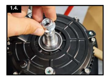
Remove the nut from the TORP motor.
