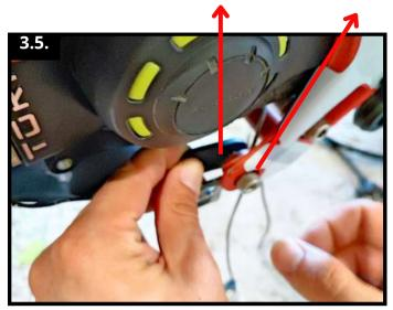
Place the black bracket on the inner side of the bike frame, then screw the bracket **loosely** to the bike frame with the M8x16 screw.
